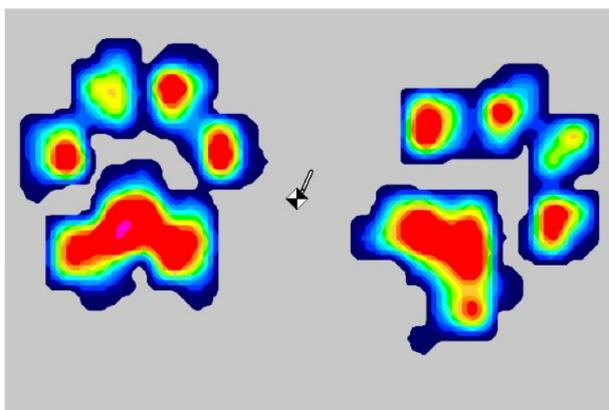
Figure 1. Peak vertical force (PVF) outline on the Tekscan mat, produced via Matscan XL software
