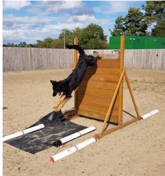
Figure 1. Scale study setup showing positioning of pressure sensing mat on landing side. The participating dog was traversing the scale at 5ft.
