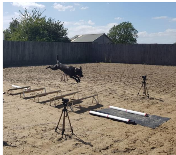
Figure 2. Long jump study setup showing positioning of pressure sensing mat on landing side.
